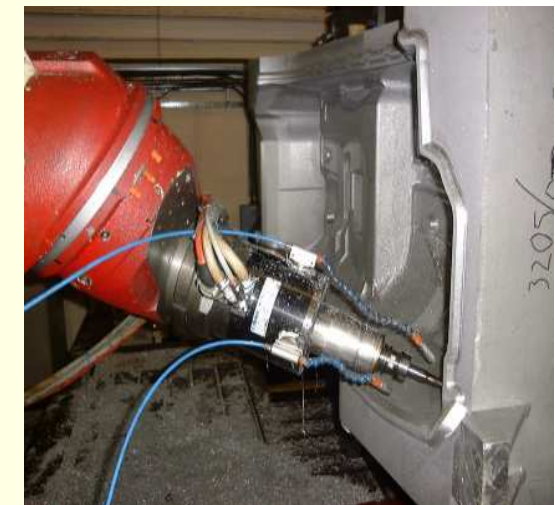
Milling of mould tool
