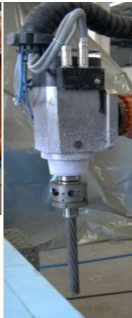
Hollow spindle and extraction for polystyrene cutting
