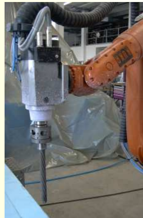
Hollow spindle and extraction for polystyrene cutting
