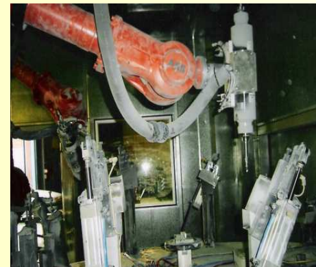
Double spindle for machining composite floor cab mouldings
