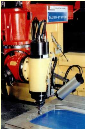
Heavy duty robot and spindle for steel cutting
