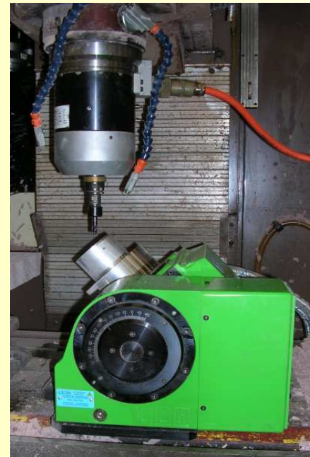
Machining centre with 2 axis table plus electro spindle for high speed 5-axis machining
